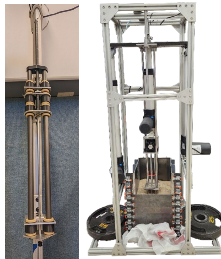
Figure 2: Single pin prototype [left] and Pin array test set-up [right].
